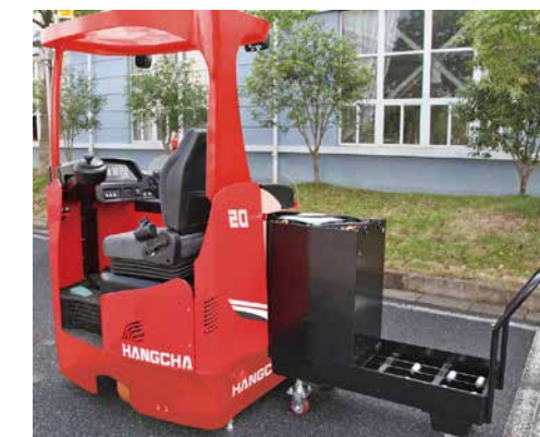
Standard configuration: Battery side roll-out + trolley(optional)
