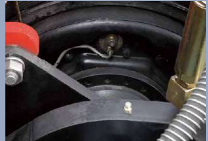
A drum brake is used, which is safer, more reliable, and easy to maintain
