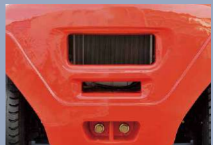
Enlarged heat dissipation channels and double-channel vents are used to ensure normal water and oil temperature. An independent hydraulic oil heat dissipater is provided, which meets the requirements of harsh operating conditions
