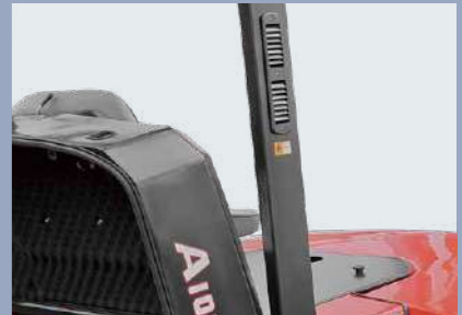
The engine's air intake pipe is provided as an independent channel in a high position to effectively prevent dust from being sucked in
